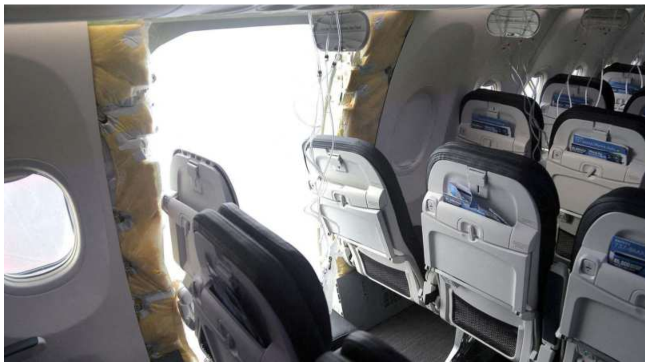
Quality control: The fuselage plug area of Alaska Airlines Flight 1282 Boeing 737-9 MAX after facing a mid-air incident in January. REUTERS
